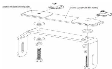
5. Using a 13mm socket and the included M8 bolts, washers, and lock washers, install your new light bar brackets as shown to the left.
