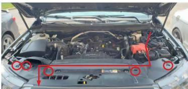
3. Route your wiring harness. We recommend routing the harness across the front of the engine bay and down the front passenger side corner to the lower grille area. This will require the core-support trim panel to be removed. It is held in place with four plastic push-rivets and two screws on the intake.
