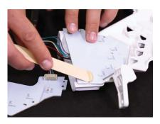
3. Place your new Diode Dynamics LED boards into position. All holes should align perfectly. Secure the new boards in place by applying epoxy or other permanent adhesive where the plastic rivets were removed. The epoxy should create a bond between the plastic rivet mounting point and the board. Use enough epoxy so that there is a bond all the way around the rivet, contacting the board fully. We recommend securing the board labeled 3 first and working your way forward.
