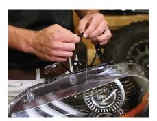
5. Run the wiring out of headlight, sealing any holes that you may create.
