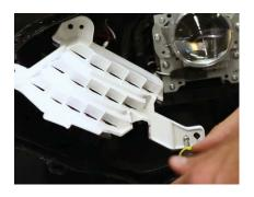
4. Once the epoxy is fully set, reinstall the white bezel to the main headlight housing using the original screws.
