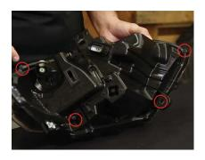
1. Open the headlight housing. To do so, remove the four screws holding the back of the headlight housing to the lens. Set the lens aside on a soft surface to avoid scratching or marring the surface.
