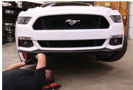
**2.** Remove the belly pan from underneath the vehicle. To do so, remove the 12 7mm screws on the outside edge, four 7mm screws on the belly pan itself, and six plastic rivets on the outside edge to remove the belly pan.
