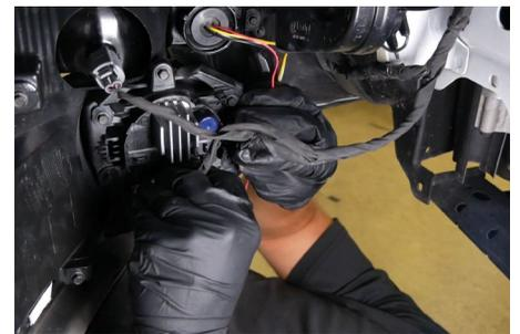
11. Plug the connector on the turn signal housing into the factory turn signal connector. Then reconnect the sidemarker and fog light connectors.
