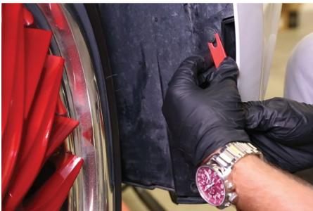
**1.** Using a plastic trim removal tool, remove the two plastic rivets holding the fender liner in place in the wheel well on both sides of the vehicle.
