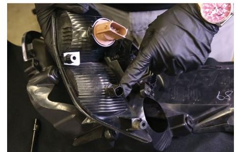
**6.** Remove the sidemarker socket from the factory turn signal housing and remove the bulb. The socket will be used with your new turn signal housing.
