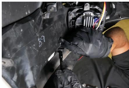
10. Reinstall the fog light bezel in the bumper, ensuring the tabs snap into place. Replace the original six screws to secure the bezel.
