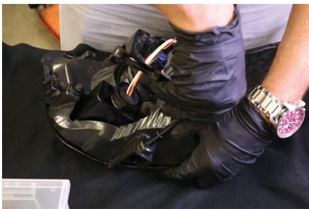
9. Install the new turn signal housing into the fog light bezel, reinstalling the three 7mm screws.
