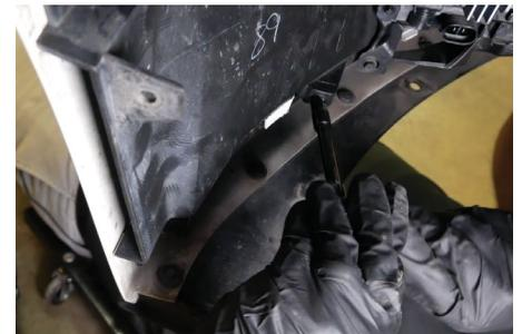
**3.** Looking at the fog light bezel, unplug the factory turn signal, sidemarker, and fog light connectors by depressing and pulling straight back. Then remove the six 7mm screws holding the fog light bezel in place.
