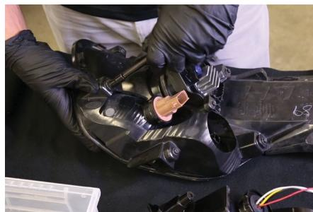
**5.** Remove the three 7mm screws holding the turn signal housing to the fog light bezel. Next, remove the turn signal housing from the bezel.
