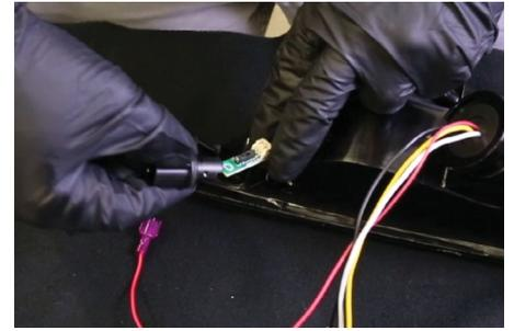
8. Once the blink rate has been set, insert the switch into the factory sidemarker socket. Reinstall the socket back into your new turn signal housing.
