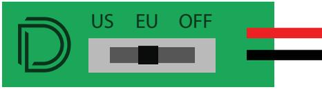
7. Using the integrated switch on your Diode Dynamics Sequential LED Turn Signal, set your desired turn signal blink rate.
