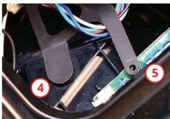
4. Place the bracket and Demon Eye into the projector housing. The pressure fitted tab should be placed in the lower hole and lock into place.
