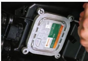
7. Route the Demon Eye wire out before reconnecting and replacing the HID ballast using the original screws.
