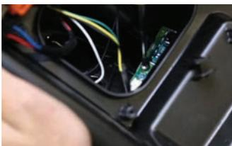
3. Unclip the HID connector and pull straight out on the HID ballast. Set it aside to provide enough working space to get inside in the headlamp. Then remove the Phillips screw holding the factory circuit board down.
