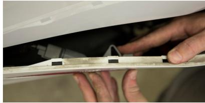
**4.** Remove the sidemarker by pressing on the clip towards the front of the vehicle, then pushing it out.
