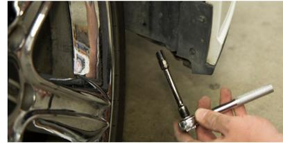
**1.** Using a 7mm socket wrench, remove the three screws in the wheel well.
