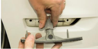
7. Twist the plug back into the new sidemarker to seal.
