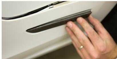
**8.** Place the sidemarker back into the bumper, clipping it into place.
