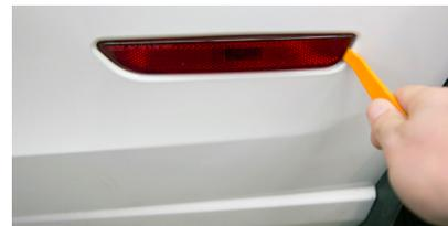
1. If you have a non-marring tool, you may be able to remove the sidemarker by inserting the tool in the backside of the sidemarker and pushing forward toward the front of the vehicle. You may then proceed to step 5.
