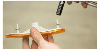
**3.** Using a 10mm socket wrench, remove the two nuts on the back of the sidemarker.
