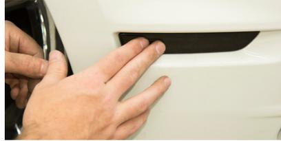
8. Place the sidemarker back into the bumper, and tighten the nuts on the rear. Do not overtighten!
