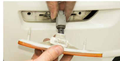
**5.** Twist the factory plug counter clockwise to remove from the sidemarker, and remove the bulb.
