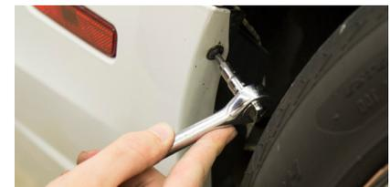
2. If you do not have a non-marring tool or are unable to remove the sidemarker, remove the three screws in the wheel well, using a small Philips screwdriver, or socket with bit.
