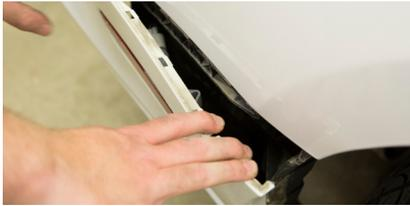
**3.** Pull back on the rear bumper, unclipping to access sidemarker.
