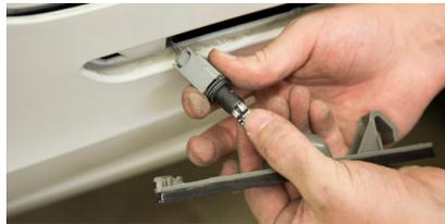
**6.** Plug the connector from your new sidemarker into the socket. Ensure you have the correct polarity by hitting the unlock button. If the sidemarker doesn't illuminate, flip the connector 180°.
