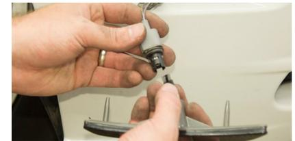
**6.** Plug the connector from your new sidemarker into the socket. Ensure you have the correct polarity by hitting the unlock button. If the sidemarker doesn't illuminate, flip the connector 180°.
