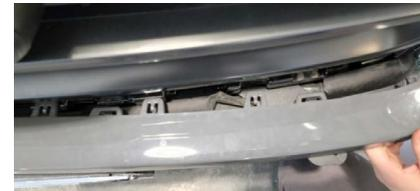
2. Repeat step one on the opposite side of the vehicle and pull the valance off entirely, starting from the outside and pulling the tabs loose working your way to the middle.
