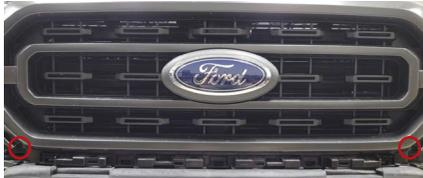
6. Remove the grille by pulling firmly away from the radiator.
