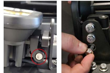
13. Mount the assembled SS5 lightbar onto the low mount brackets using one 10mm bolt on each side. Rotate the lightbar upward, exposing the end bolt in the pivot mount. Tighten the pivot mount bolt with a 5mm Allen wrench and rotate the lightbar back down to install the other two 10mm bolts.
