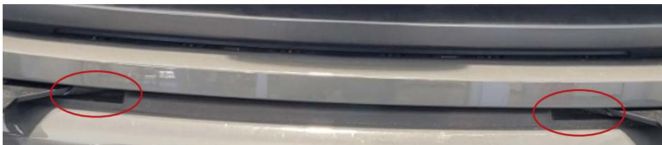
8. Route the included wiring harness through the opening in the rubber seal, next to the bracket. The connector will not fit through the opening with the plastic valance installed.
