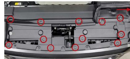
3. Remove the trim panel on the radiator core support by pulling out the 13 tree clips securing it.
