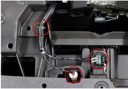
4. Disconnect the harnesses near the hood latch and remove the clip securing the harness to the grille.
