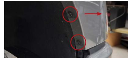
1. Using a 7mm socket, remove the the screws securing the fender liner to the upper bumper valance and pull the sides of the valance loose from the fender well and the fender.
