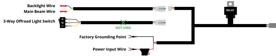
15. Locate the auxiliary switch wiring near the battery. Access the owner's manual in the head unit and determine what wire color you will connect to based on the amperage rating. Connect the yellow wire for the main beam to an auxiliary switch wire. Using wire strippers, remove enough insulation to make a good connection. Insert the wire into the butt connector and crimp it to secure the connection.
