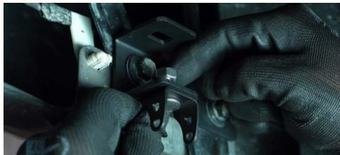
2. Install the universal pod bracket onto the reverse light bracket using the provided hardware. Make sure that the curved portion of the bracket is facing towards the rear of the vehicle.
