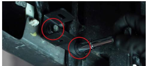
1. Using a 13mm socket and ratchet, remove the factory bolts shown in the picture above on the underside of the truck bumper. Then install your new reverse light bracket onto the vehicle using the factory bolts.
