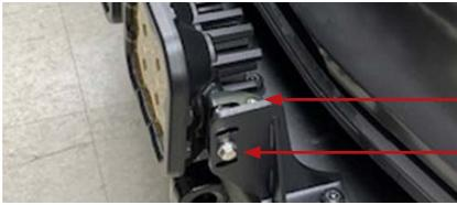
4. Mount the assembled SS5 lightbar onto the brackets with provided the M6 flange screws.
