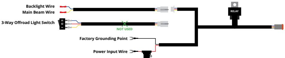
5. Locate the auxiliary switch wiring above the grille. Access the owner's manual in the head unit and determine what wire color you will connect to based on the amperage rating. Connect the yellow wire for the main beam to an auxiliary switch wire. Using wire strippers, remove enough insulation to make a good connection. Insert the wire into the butt connector and crimp it to secure the connection.
