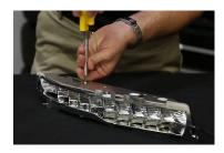
7. Reinstall turn signal housing into main headlamp housing. Run RGBW ribbon cable out of headlamp, along with the 2-wire connector, sealing any holes that you may create. If desired, plug the sidemarker into the factory driver board. Using the alignment pins, set the unit into place. Once complete, replace the torx screws and headlamp lense.
