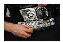
1. Access the factory LED panels by removing the screws holding the turn signal assembly in place. Remove the chrome reflector unit by depressing the clip on the back of the driver.
