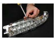
2. Then, remove the torx screws holding the metal bracket to the chrome reflector. Once complete, separate the chrome reflector from the metal bracket. Bring the metal bracket to a clean area away from the chrome reflector.
