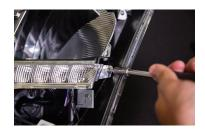
4. Remove the screw holding the turn signal reflector in place on each side and disconnect the factory harness. Then remove the housing and set it aside.
