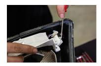
6. Remove the light pipe from its retaining clip by gently pulling the pipe away from the board until the tabs on the pipe release from the clips. Repeat for the other side to fully remove the light pipe.
