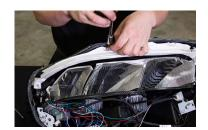
9. Secure the upper optics shroud back in the retaining clips one side at a time.
