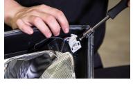
7. With both optics shrouds and the turn signal reflector removed, remove the four T20 screws holding the factory boards in place.
