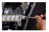
11. Reinstall the turn signal reflector by reconnecting the factory harness and reinstalling the screw that was removed in step 4.
