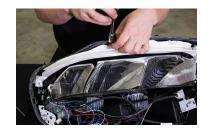
5. Remove the five T20 screws holding the upper optics shroud and light pipe in place.
