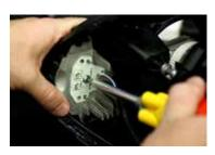
4. Using the alignment tabs, place the new board into place and replace the original retaining screw. Next, replace the black alignment bracket using the original screws. DO NOT OVERTIGHTEN.
