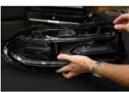
7. Using the alignment tabs, reinstall the black bezel. Once complete, replace the original torx screws and headlamp lense. Repeat for other headlamp.
