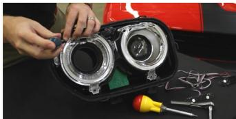
1. After opening the headlights, remove the factory LED panels by removing the screws holding the main bezel in place. Then remove the screws holding each ring and LED panel underneath to the housing.
