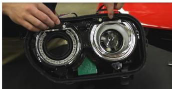
3. Place the new Diode Dynamics LED Boards into position, running the wires behind the bezel and out of the headlamp, sealing any holes you may create.
