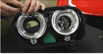
4. Using the alignment tabs and original screws, align the ring and screw back down, securing the LED boards. **DO NOT OVERTIGHTEN.** Replace the headlamp lens and repeat for the other side.
