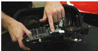
2. Remove the main bezel. Unclip the wire connectors and remove the factory LED panels.
