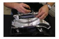
1. With the headlamp open and lens removed, remove the six T20 screws holding the DRL and turn signal reflectors in place.
