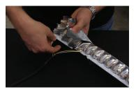
5. Using the included wiring harness, connect the harness to the boards. It doesn't matter which connector gets connected to each board.
