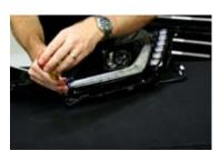
6. Replace the main black bezel and secure it using the original screws.
