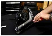
1. Remove the three Torx T20 screws that hold the main black bezel in place. Remove the black bezel and set it aside.
