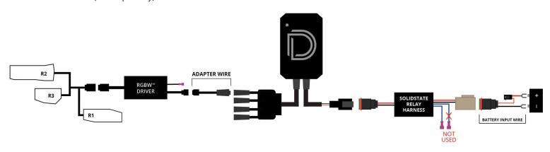
IMPORTANT: DO NOT plug the LED panel directly into controller without the driver. The LEDs must be plugged into driver first to control the power.
