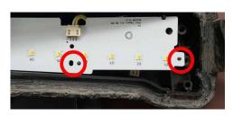
13. Install your new LED board into the lamp housing, aligning the tabs. Then reinstall the original screws and optic. Reinstall the black shroud. Once complete, repeat the same process for the other lamp.
