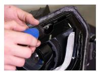
1. Remove the six T20 torx screws holding the black bezel in place, including the screw on the backside of the housing. Set the bezel aside.
