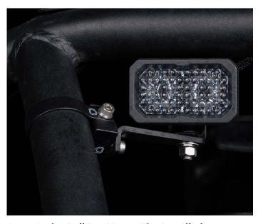
Stage Series Roll Bar Mount Kit - Installed
