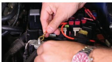
7. Connect the module from the wiring harness to the spade connectors on the fuses
