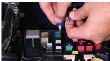
6. Reinstall the fuses back into the fuse box, ensuring the 15A fuse goes into the high beam slot (fuse 7) and the 30A fuse goes into the low beam slot (fuse 6).
