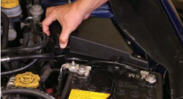
1. Access the fuse box located in the engine bay. Remove the fuse box cover and set it aside.
