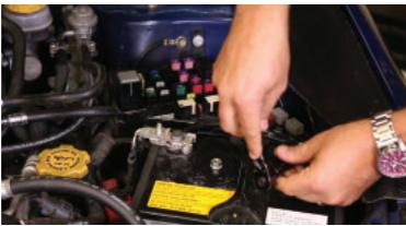
2. Remove the 12mm nut and loosen the 10mm nut on the battery posts.
